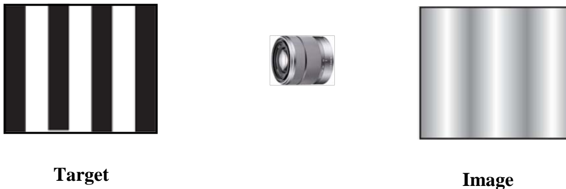
Figure 2. Schematics showing the contrast reduction in the image compared to the object
